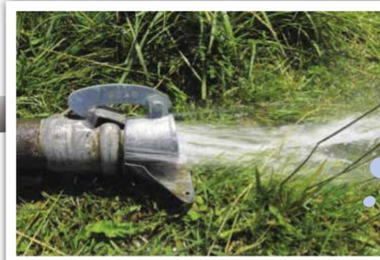
And how about an end plug leaking – any guesses? It loses 10 gpm, \$46 per year if pumped from a canal and \$132 per year if pumped from a well. And that's 2.76 acre feet of water you could have used in production somewhere else.
