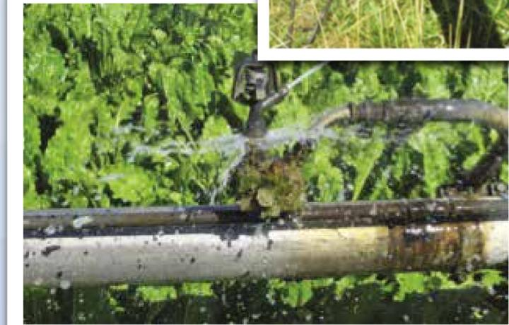
This leaky nozzle will lose 2.3 gpm, and cost \$11 per year if pumped from surface water or \$30 per year if pumped from a well. This nozzle alone loses .63 acre feet per year. How many leaky nozzles are on your farm?
