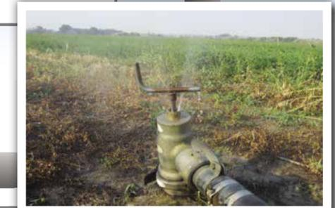
This baby geyser seems harmless enough. Yet even at a rate of 0.5 gpm, it results in a loss of \$2.32 per year if water is pumped from a canal and \$6.60 per year if pumped from a well. And you'll still lose .14 acre feet of water.
