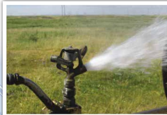
When a sprinkler head blows out altogether, it's like running a pressure sprayer at full throttle. This one lost 20 gpm, and will result in a loss of \$93 per year if pumped from surface water sources, and \$265 per year if pumped from a well. Over a season, it will lose 5.52 feet per acre.
