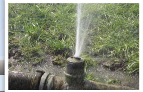
And who hasn't seen the geyser spray before? This spray, although seemingly minor, loses 4.6 gpm. If lifting water from a 30-foot drop, losses would total \$21 per year in electrical fees. If pumped from a well 300-feet deep, electrical fees lost would equal \$61 per year, and water losses will equal 1.27 acre feet.
