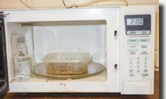
You may continue drying in half-minute time settings as long as the glass of water is kept three-quarters full. If the forage chars, use the weight previous to the burning.
